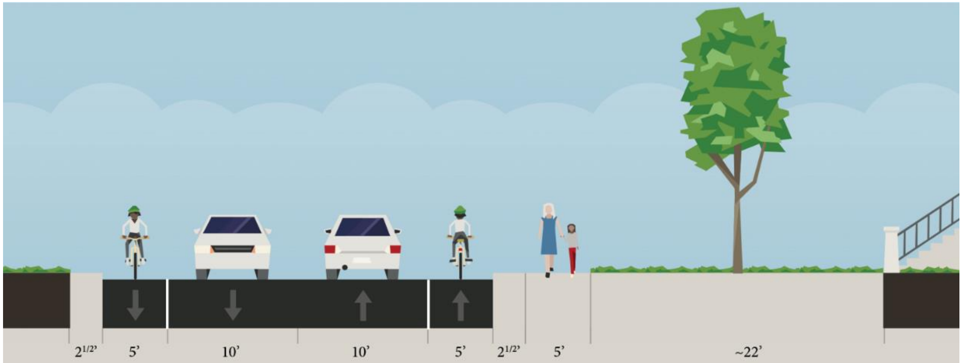
Exhibit A – Little Kate Road Existing Cross-Section
