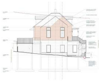
Historic fabric to remain on restored roof (painted wood siding)
