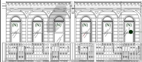
Figure 5: Proposed windows on the second level of the front facade of the Historic Structure.
