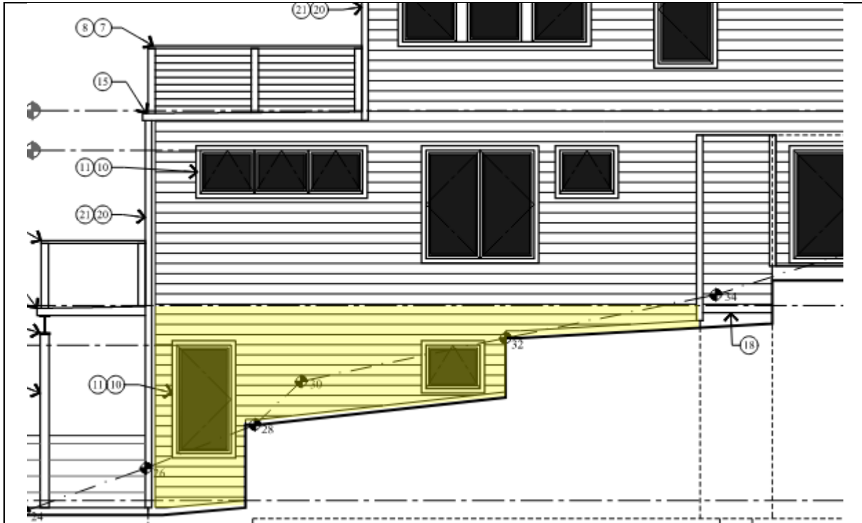
Figure 2: Area shaded in yellow is the exposed foundation clad in additional siding material
