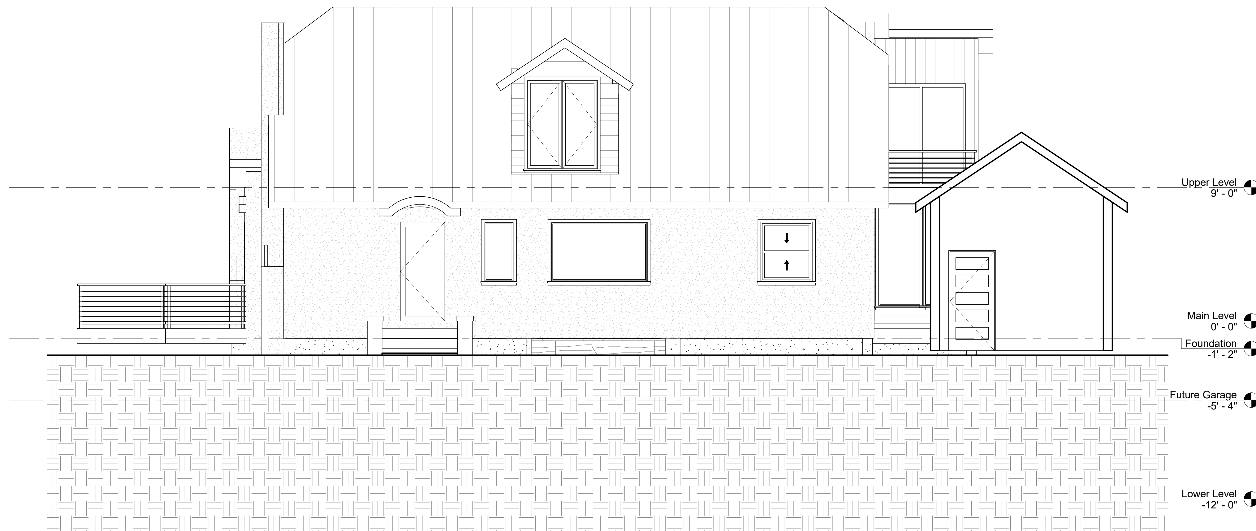
2 Exterior Elevation - West - Same Spot 1/4" = 1'-0"
