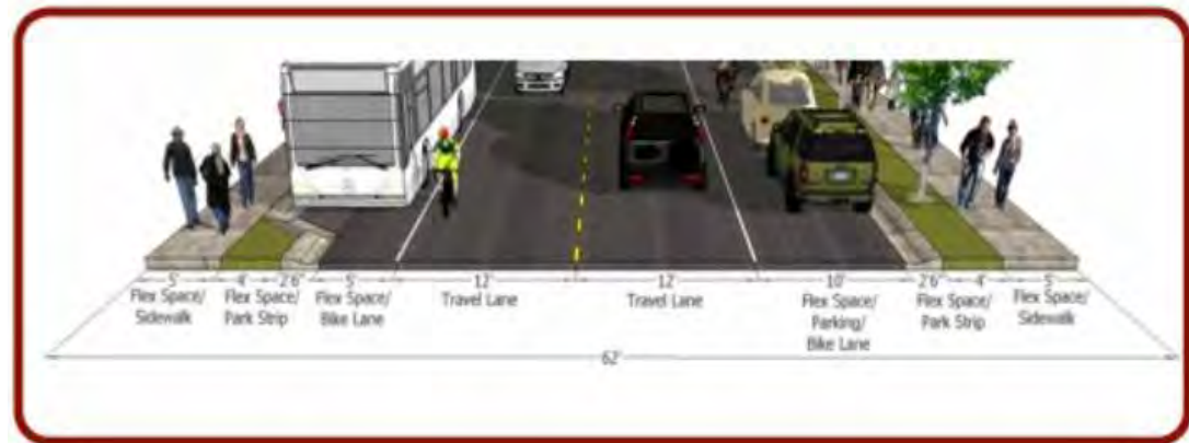
The 2011 Park City Traffic and Transportation Master Plan reinforces the City’s goal to create complete streets. Above: Major Residential Collector cross section from PC TTMP.
