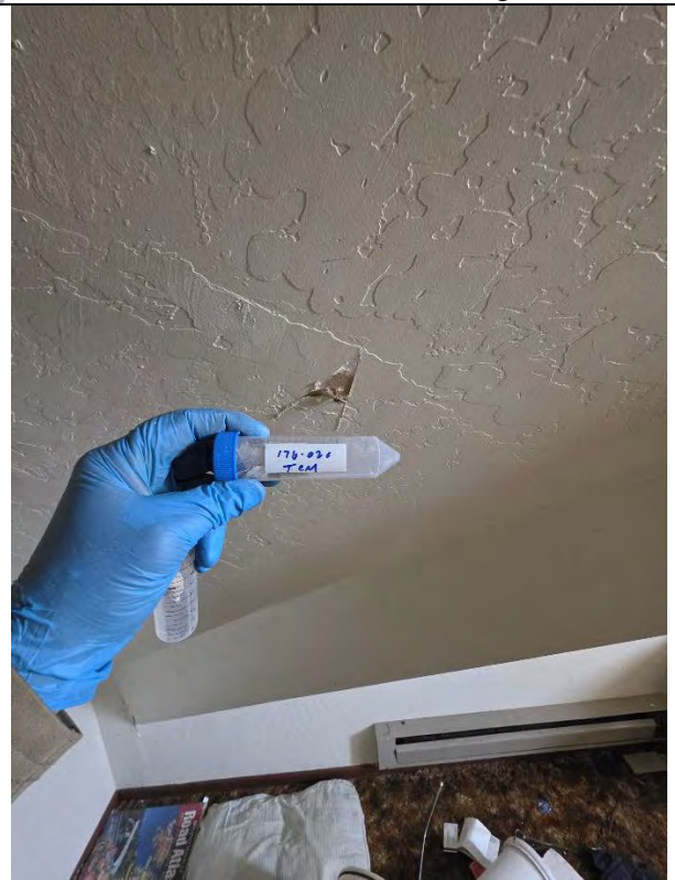
176 – 02C Textured Wall/Ceiling Material
