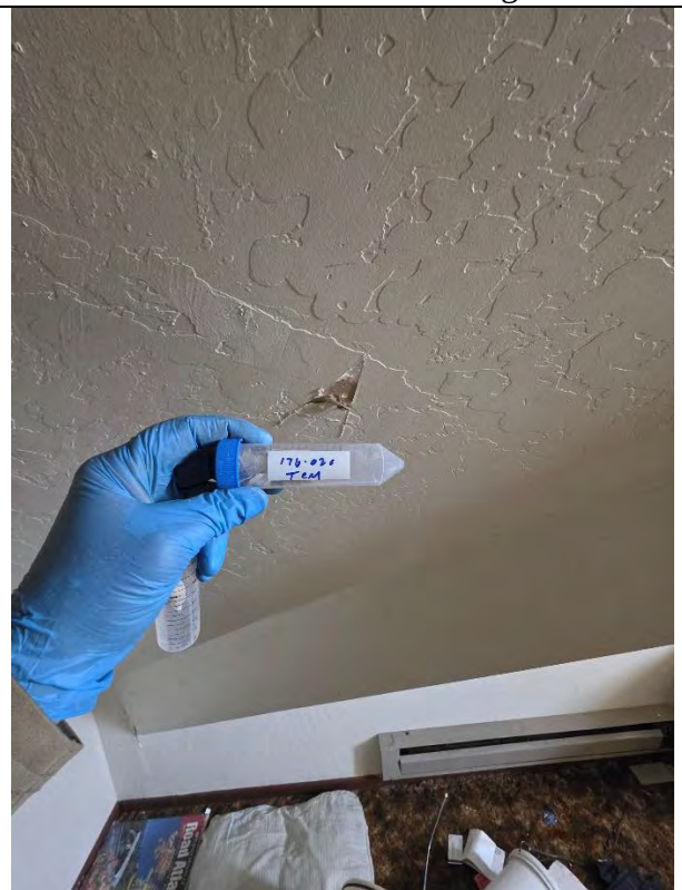
176 – 02C Textured Wall/Ceiling Material
