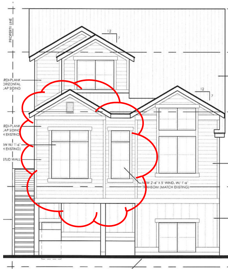
HDDR Modification plans showing proposed enclosed deck (changes shown in red bubble) – east elevation
