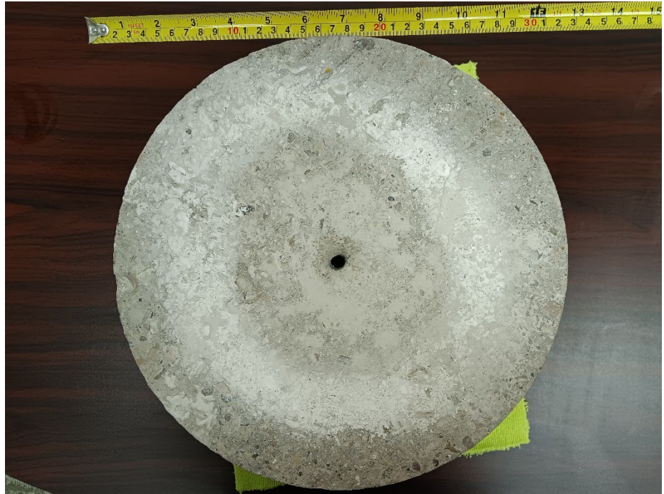
Photograph 1: Concrete core B-1 taken from the slab-on-grade parking area.
