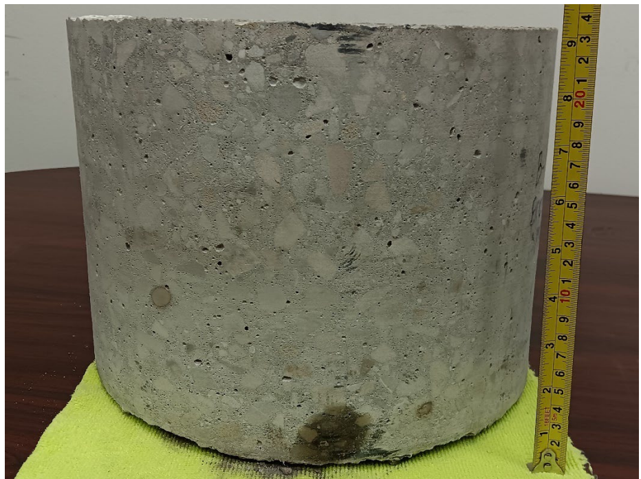
Photograph 2: Concrete core B-1 taken from the slab-on-grade parking area.
