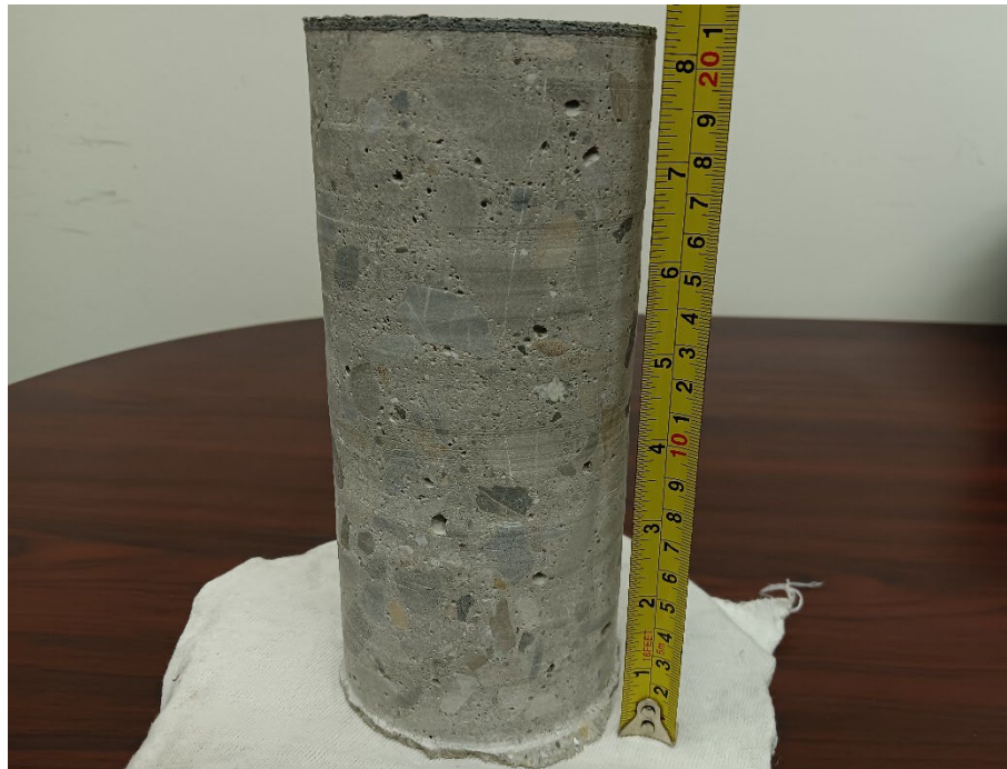
Photograph 8: Concrete core C-3 taken from the southwest corner of the upper deck of the parking structure.
