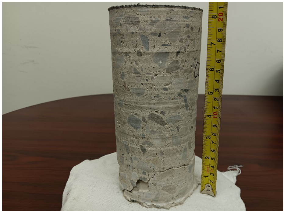
Photograph 6: Concrete core C-2 taken from the central portion of the upper deck of the parking structure.
