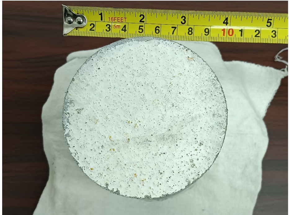
Photograph 15: Concrete core C-7 taken from the northwestern portion of deck 2S in the parking structure.
