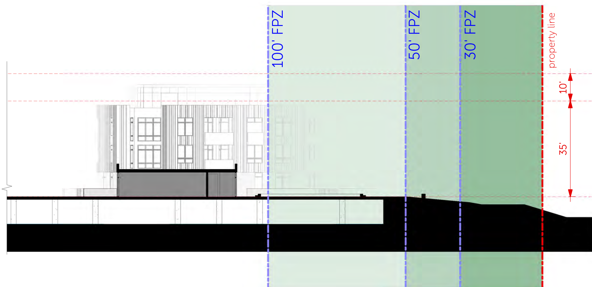
3 Proposed Connector D/C Section - Kearns Blvd. SCALE: 1" = 20'-0"
