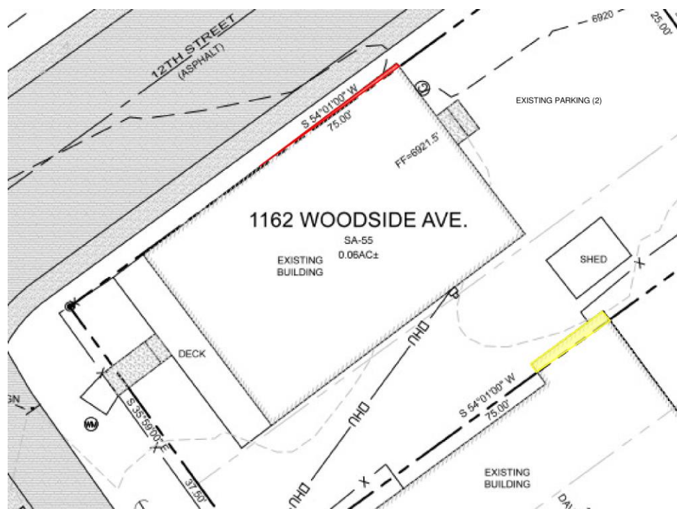
Figure 1: Property survey with encroachments highlighted:
