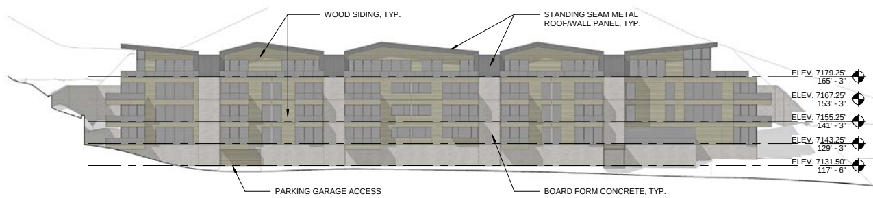
② SOUTH ELEVATION - PHASE III 1/32" = 1'-0"
