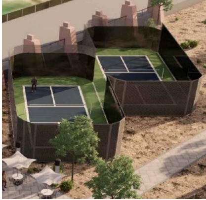
Figure 6. Illustration of pickleball courts with noise-mitigating fencing around the play area
