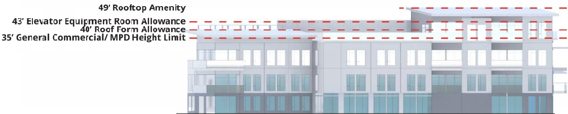
South Elevation - Fourth Floor (MPD) - Rooftop Amenity 1" = 20' - 0"
