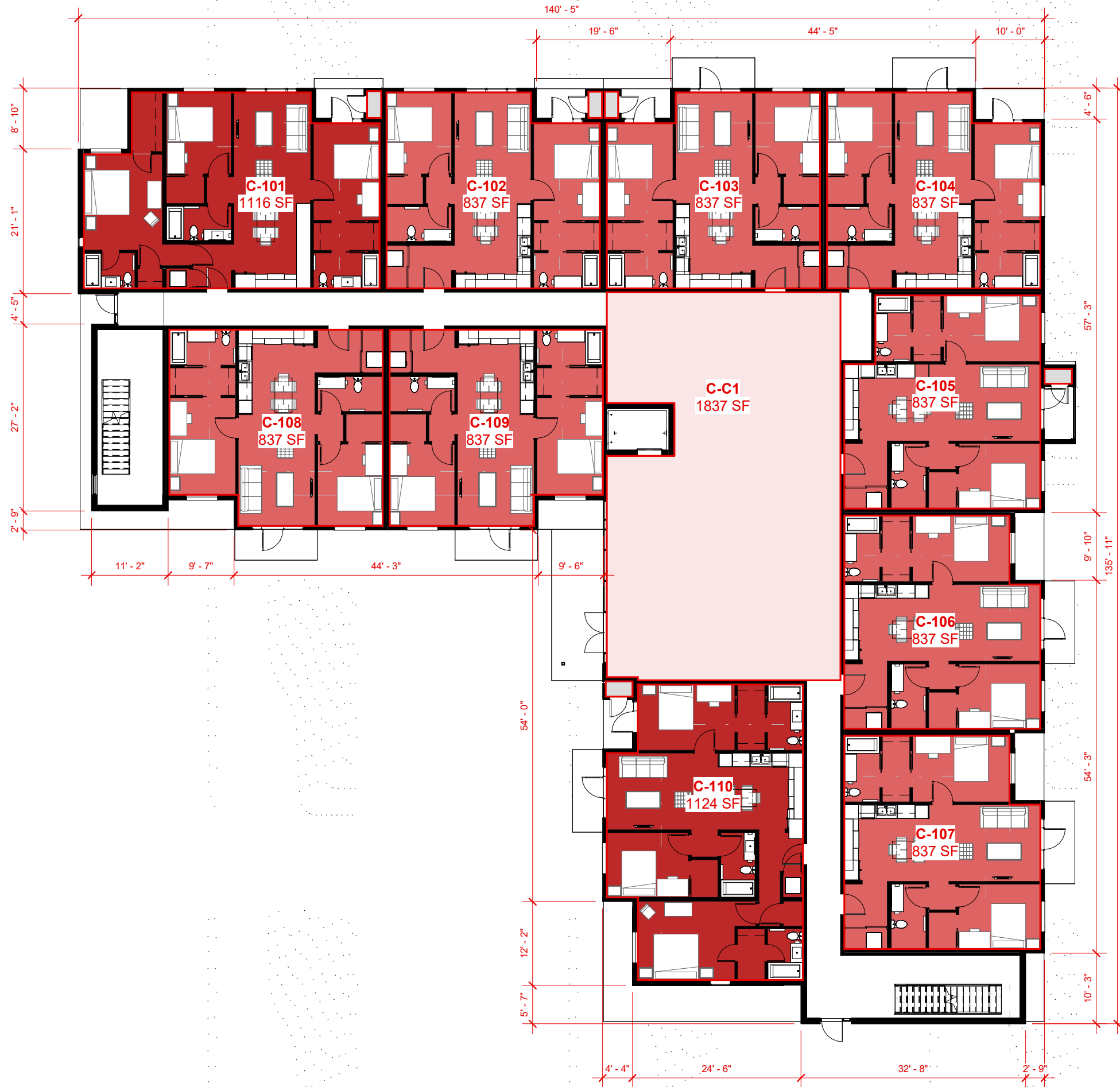
Building C - Level 1 SCALE: 1/16" = 1'-0"
