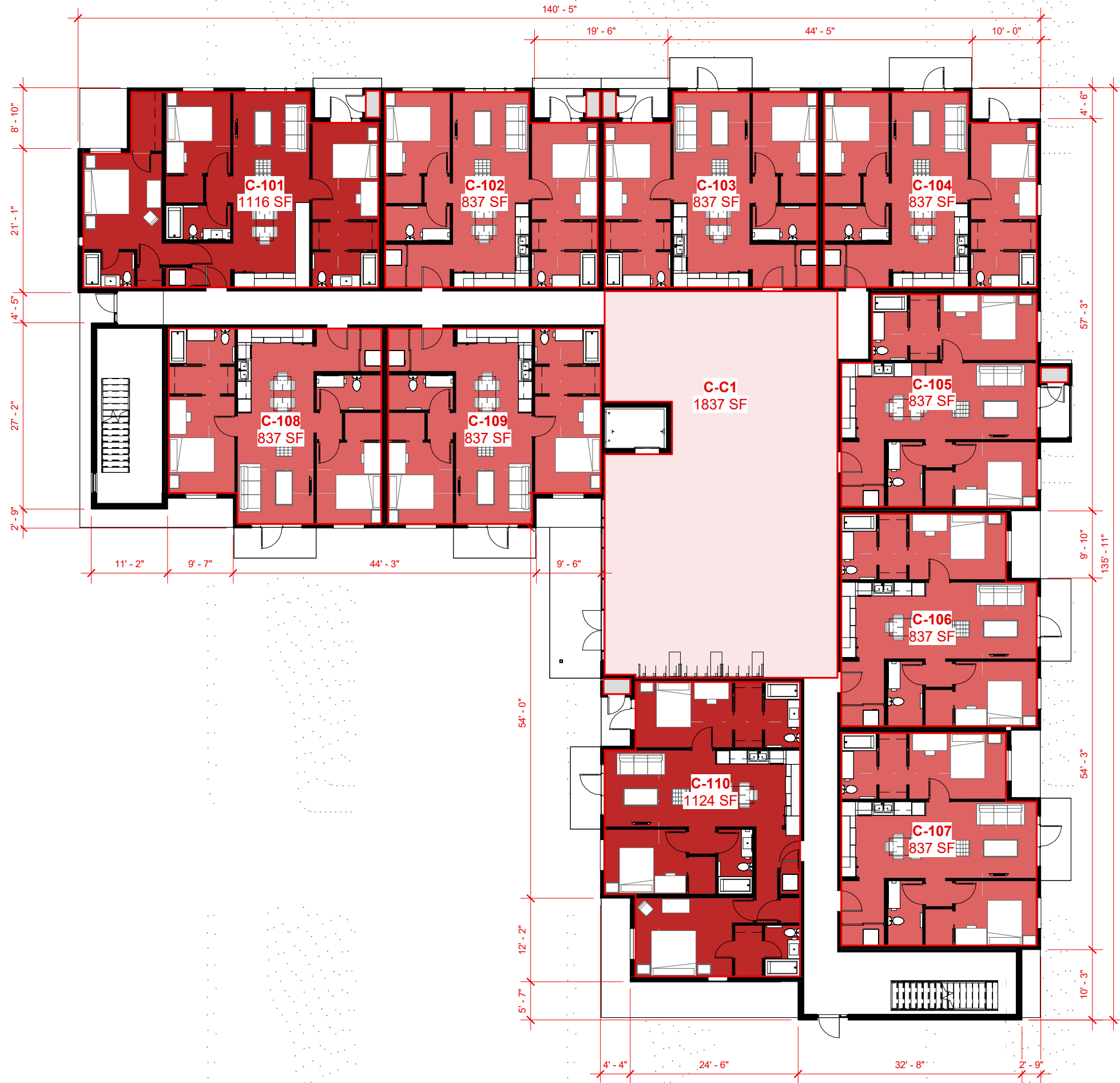
Building C - Level 1 SCALE: 1/16" = 1'-0"
