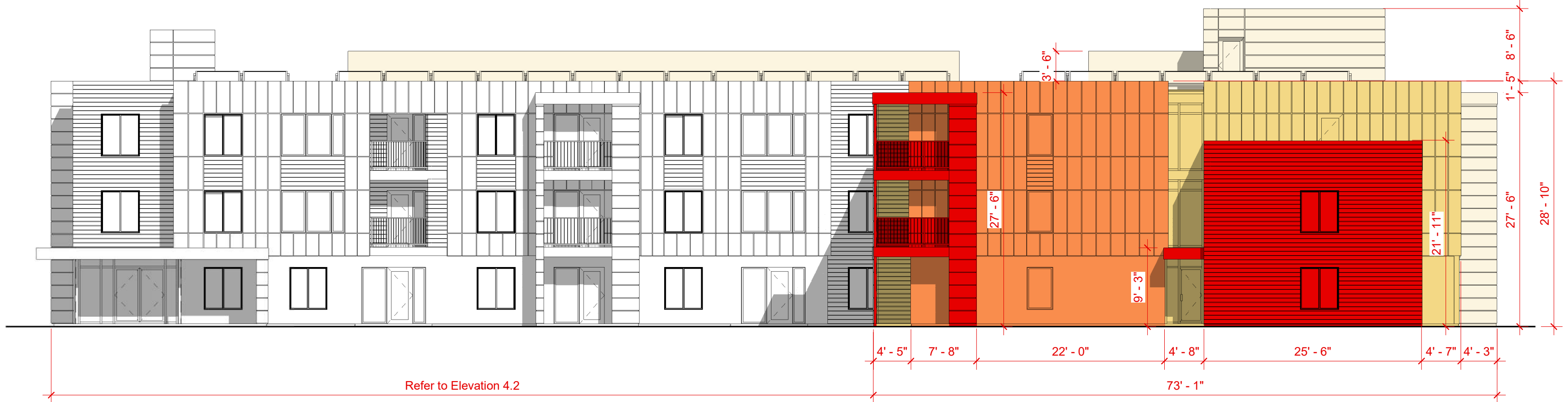
Elevation 4.1 Facade Variation
