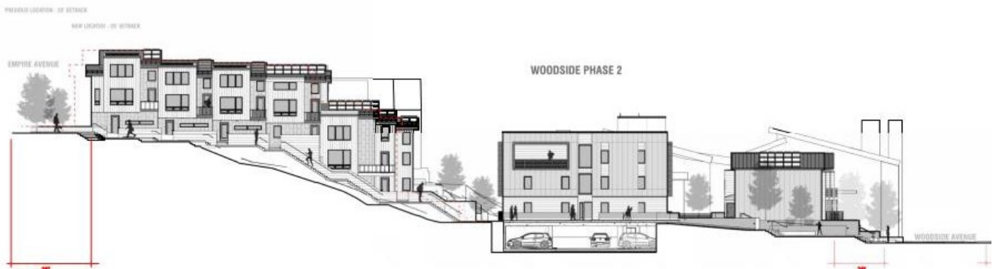
Figure 1: Excerpt from Exhibit A (Sheet C102). Elevation drawing of the proposed Setback reduction to the Zone Required Setback.
