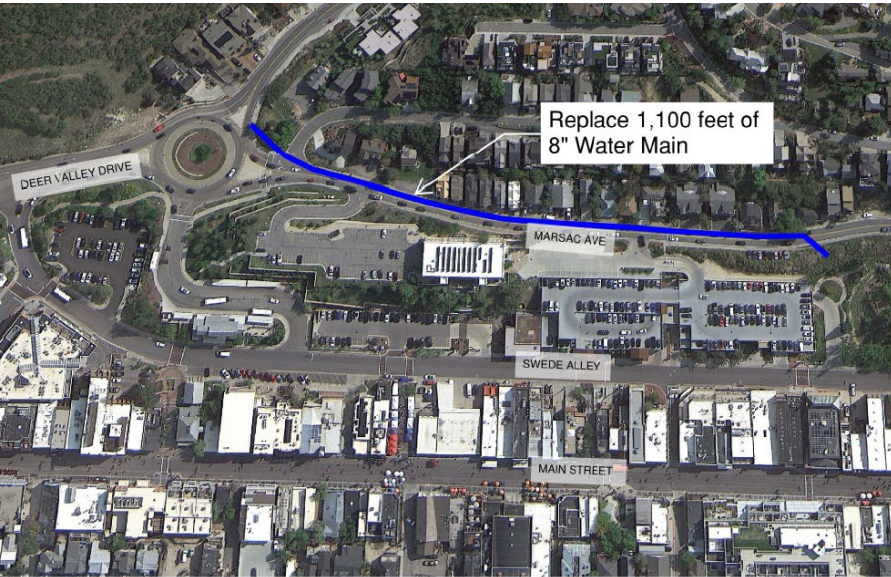
MARSAC AVENUE WATER LINE REPLACEMENT
