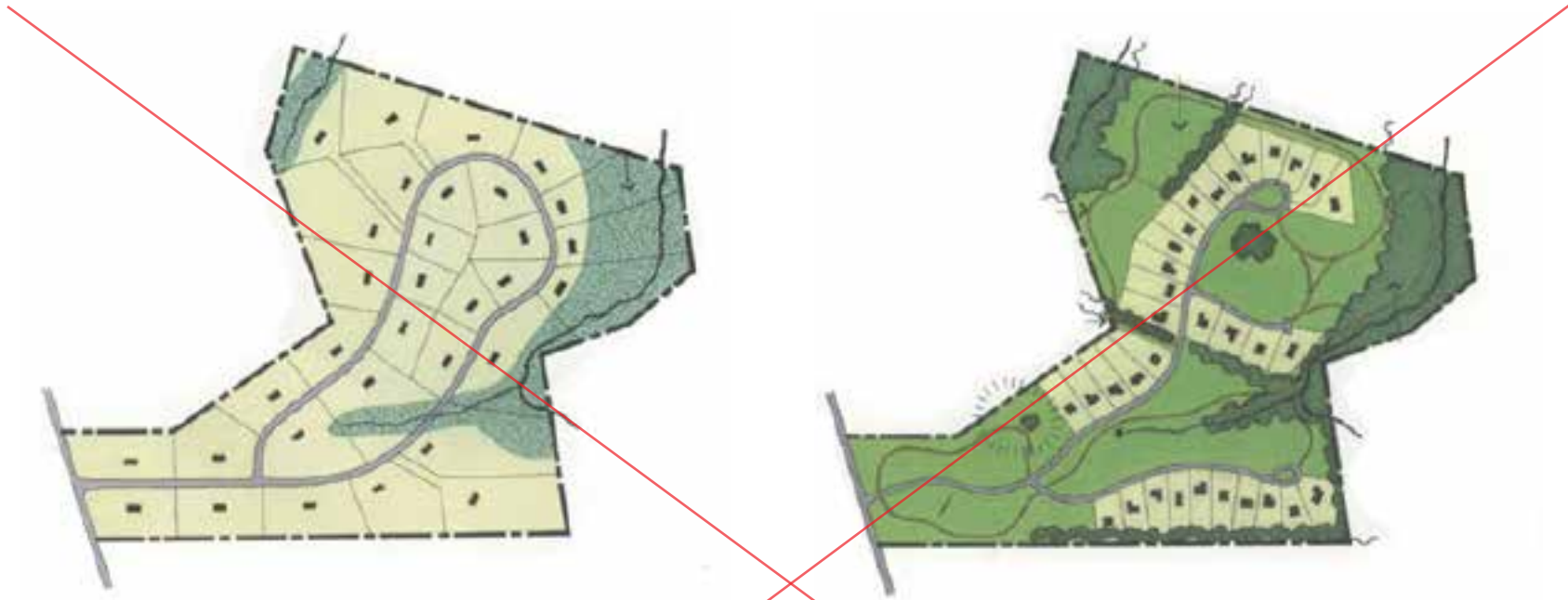
The side-by-side comparison of a traditional subdivision and a conservation subdivision design exemplifies how the natural setting may be further preserved through building pads and clustered lots.
