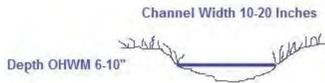
Figure 4 – OHWM – Lower Perennial Channel at Existing Road Crossing
