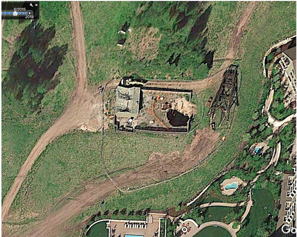
2015 Aerial photo showing extent of mine shaft collapse
