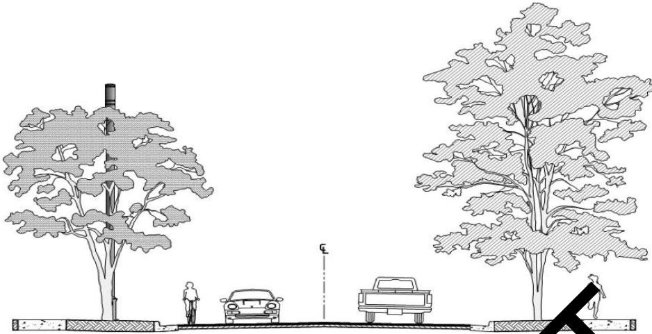
Figure 6-3: Freestanding Pole SWF in City ROW
