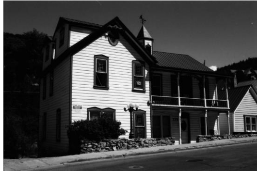
176 Main Street: Incompatible dormers located on secondary façade, and cupola added to the roof ridge of the façade.
