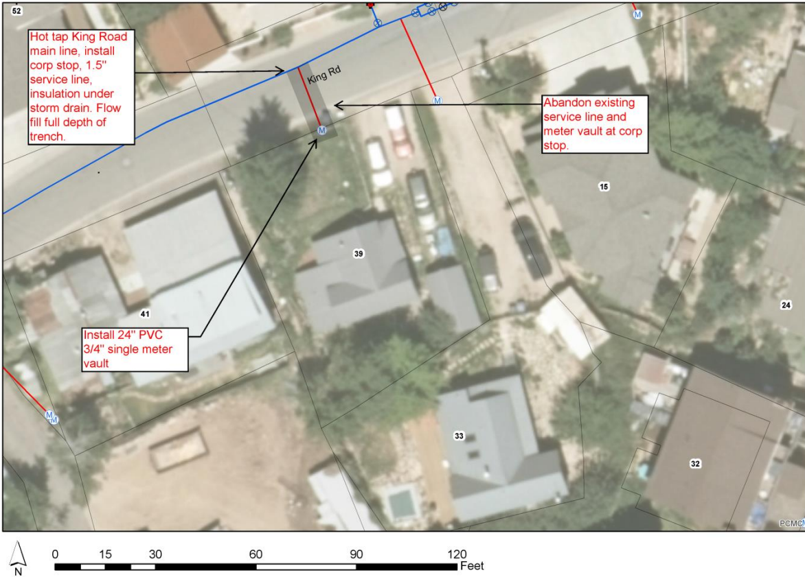
39 King Road Service Line Replacement - Site Plan
