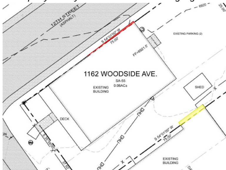
Figure 1: Property survey with encroachments highlighted:
