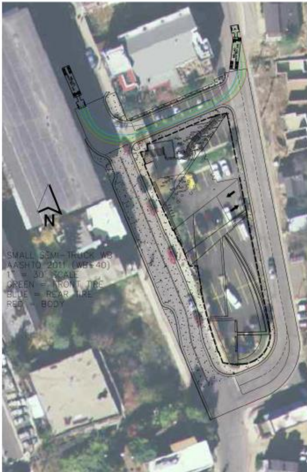
Figure 2: Large Truck Turn Around to Swede Alley
