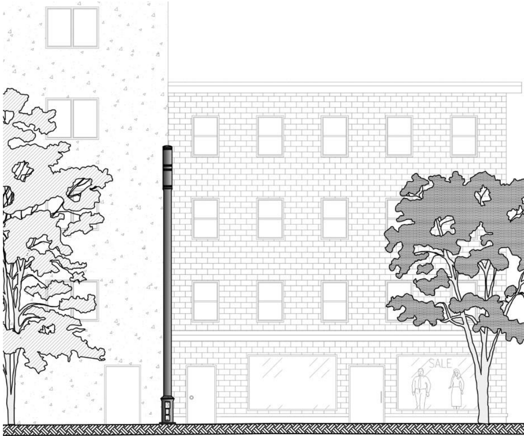
Figure 6-7: Small Cell In Commercial Area
