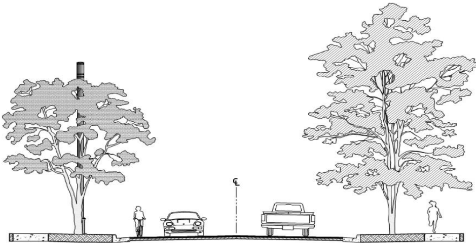
Figure 6-3: Freestanding Pole SWF in City ROW
