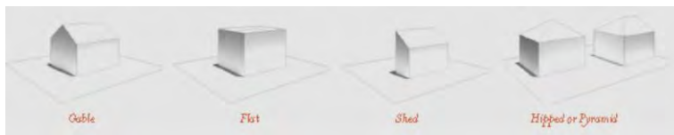
Samples of appropriate roof forms
