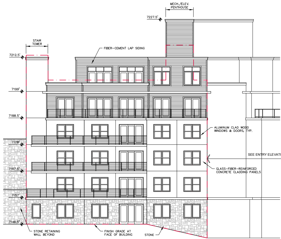
NORTHEAST ELEVATION - SOUTH WING
